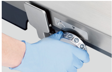
Step 1: Rotate the function icon to the position indicated by the arrow.
